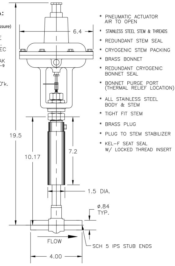
1/2"IPS CRYOGENIC VALVE W/PNEUMATIC ACTUATOR
