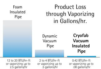
\*Data based on 100 ft. of 1" inner with liquid nitrogen.
